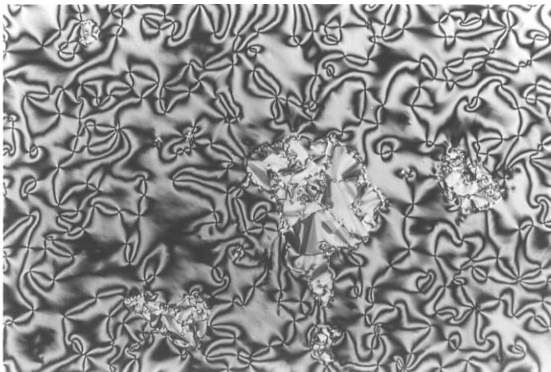
Figure 3. Polarizing microscope photograph of hexakis(4-(4'-octyloxy)biphenoxy)cyclotriphosphazene (HOCP, n = 8 ) at 453 K in the first cooling process.
